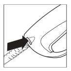
→ STEP 4: Connect the detergent suction tube to the pressure washer.
